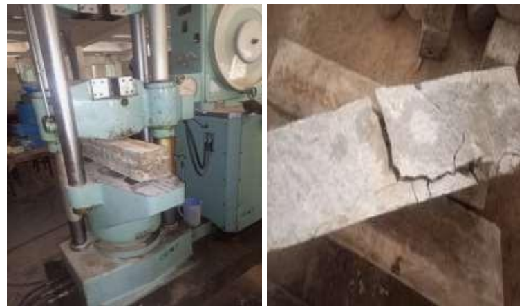
Figure 3 Pictures of Flexural Beams Subjected to Bending Using Universal Testing Machine (UTM)
